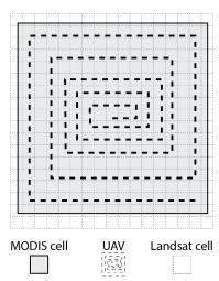
Figure 2: Conceptual drawing of the UAV flight plan with regards to a MODIS and Landsat cell.
