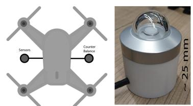
Figure 1: A schematic of how the prototype mount will be designed and implemented (left). The image on the right is the PR1 pyranometer (Kipp and Zonen).
