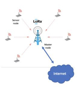
Figure 1. Conceptual deployment of Sensor Nodes using LoRa to communicate with a Master Node that pushes data to the Internet via satellite modem.
