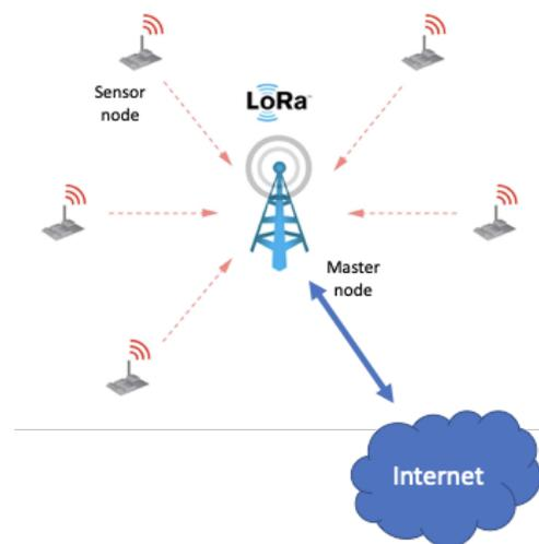
Figure 1. Conceptual deployment of Sensor Nodes using LoRa to communicate with a Master Node that pushes data to the Internet via satellite modem.
